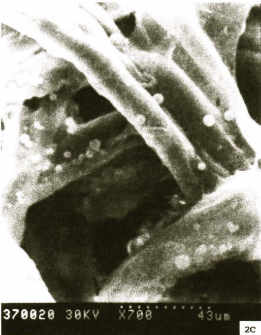
Fig. 2. Scanning electron photomicrograph demonstrating smoke particles trapped after laser plume had been filtered through A) paper mask B) cotton mask C) cotton mask at higher magnification. Note that there were still quite a number of spherical shape particles, which represented the particles passing through surgical mask, many of which were in the alveolar hazard zone.
