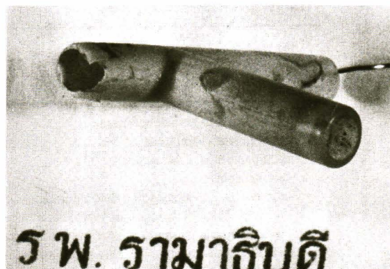
Fig. 2. The T tube that was burnt during the operation.
