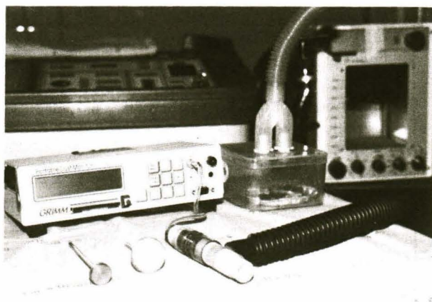
Fig. 1. Ventillog lung machine on the right, nasal with pharyngeal model and airway passage attached to the laser evaporation box at the center, laser diode portable dust monitor and accessories on the front left, laser smoke particle generator on the left.
