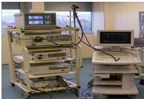
Fig. 1 Endoscopic ultrasound instruments (Pentax EG38UT and Hitachi EUB6500)
