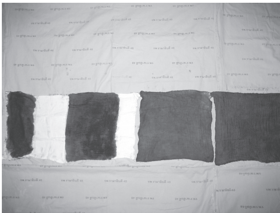
Fig. 1 Blood absorption characteristics of a dry 30 × 30 cm abdominal swab. For this particular type, 25 ml of blood saturates about 50% of the surface area, 50 ml of blood saturates about 75% of the surface area, 75 ml of blood saturates the entire surface, and 100 ml of blood will saturate and drip from the sponge
