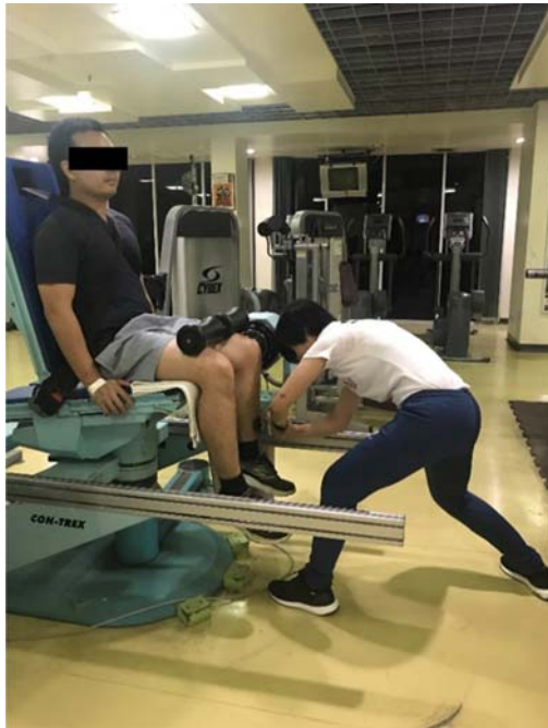
Figure 2. Hand-held dynamometry in a sitting position.
