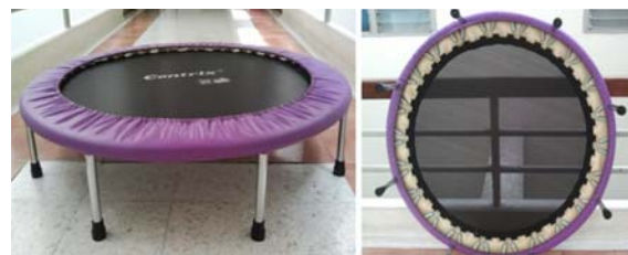
Fig. 1 Mini-trampoline compound: diameter of 1.22 m, stand all steel 8 pieces and height of ground 21.5 cm, pick weight 100 kg and spring 44 pieces.
