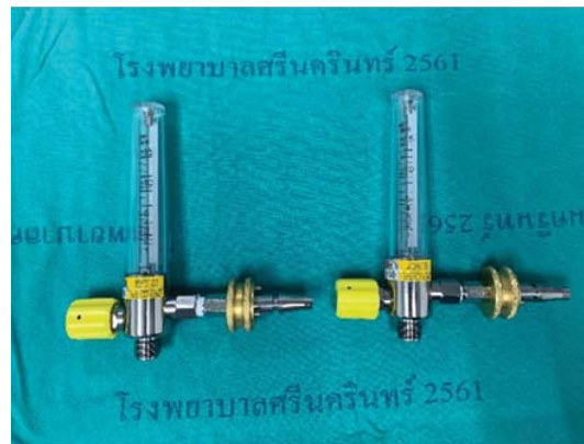
Figure 4. Ambient air flow meter with capacity of 15 liters per minute, total 2 units.
