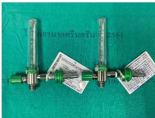
Figure 3. Oxygen flow meter with capacity of 15 liters per minute, total 2 units.
