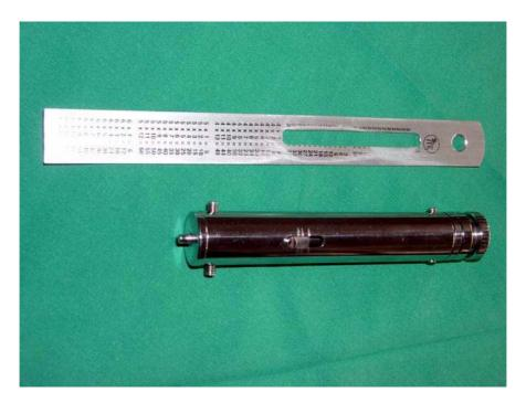
Fig. 1 Dermographometer (James and Warin's modification)
