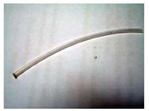
Fig. 1 The polyethylene tube, prepared by heating one end and flattened to flare it out
